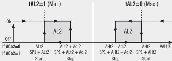
AC02 is the Alarm 2 configuration parameter
