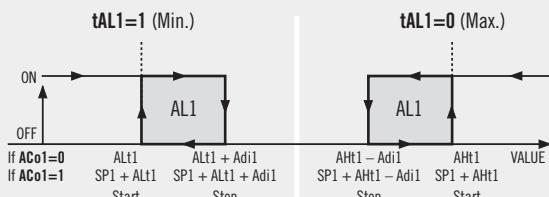
AC01 is the Alarm 1 configuration parameter
