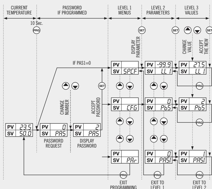
**REMARK:** If no key is pressed for 25 seconds in either of the previous steps, the controller will automatically return to the CURRENT TEMPERATURE display status without modifying any of the parameters values.
