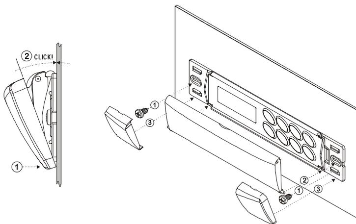
**7.3 MOUNTING WITH KEYBOARD COVER OPENING UPWARD**
