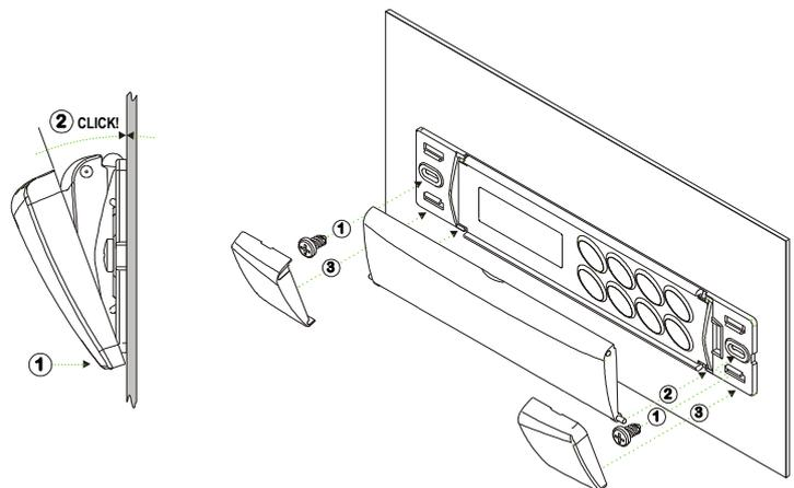
**8.3 MOUNTING WITH KEYBOARD COVER OPENING UPWARD**
