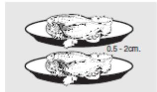
**c)** Position trays inside the tray compartment as far as they will go, as close as possible to the evaporator.
