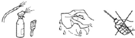
Clean with water and non-abrasive neutral detergents. Rinse with a damp cloth or sponge, or with a gentle jet of water (no stronger than mains pressure). Do not use pointed or abrasive instruments to scrape appliance surfaces. **NEVER USE ABRASIVE FLUIDS, SOLVENTS OR THINNERS**
