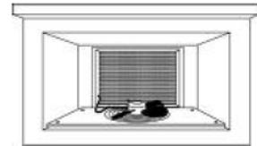
Periodically, provide to clean the evaporator, using nebulized hot water at low pressure, and addressing the water throw on the evaporator battery
