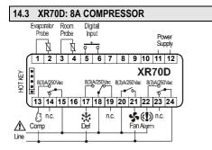
24Vac/dc supply: connect to the terminals 11 and 12. 120Vac supply: connect to the terminals 11 and 12. 230Vac supply: connect to the terminals 11 and 12.
